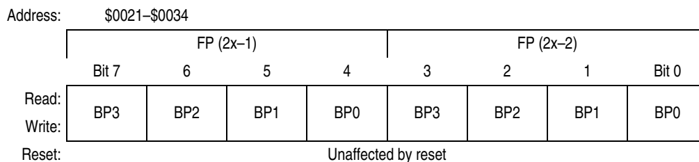
Figure 10-6. LDC Data Registers
