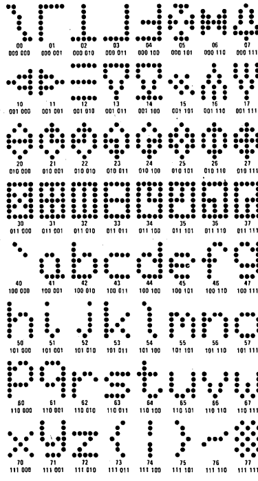
FIGURE 4. MM5240AE Horizontal-Scan ASCII-7 Lower-Case Graphic and Control Symbol Subset
