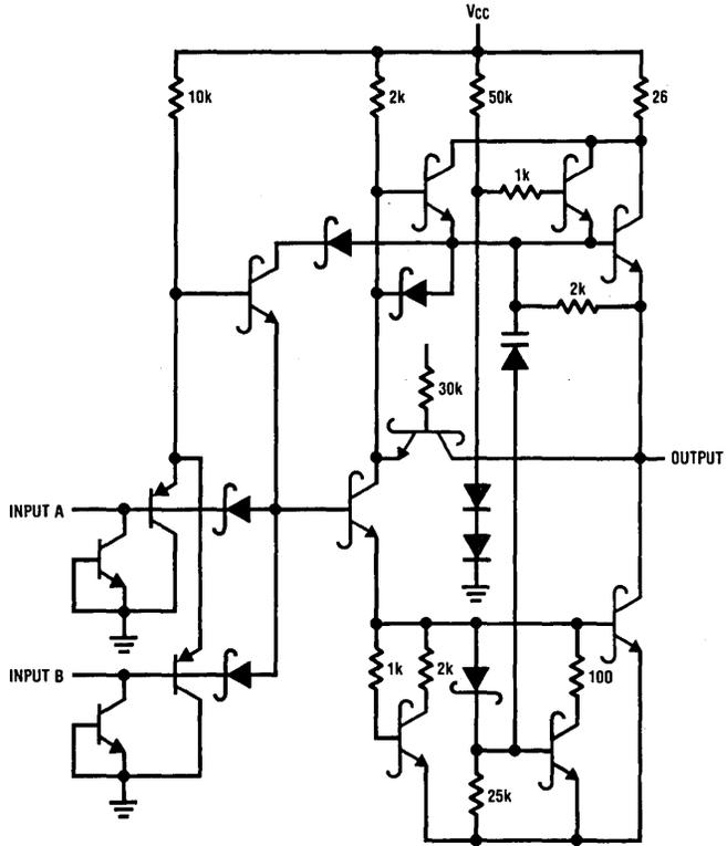
FIGURE 6. DM54AS00/DM74AS00
