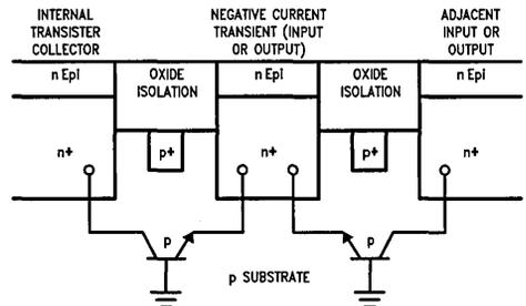
FIGURE 6. Parasitic Failures Modes
