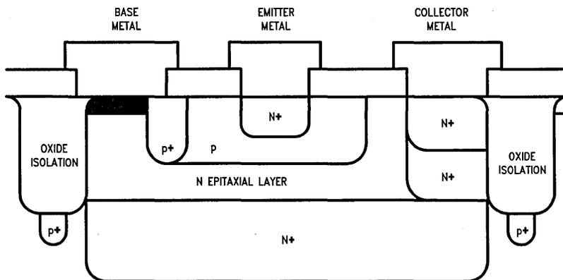
FIGURE 12. Cross Sectional View of Oxide Isolated Transistor
