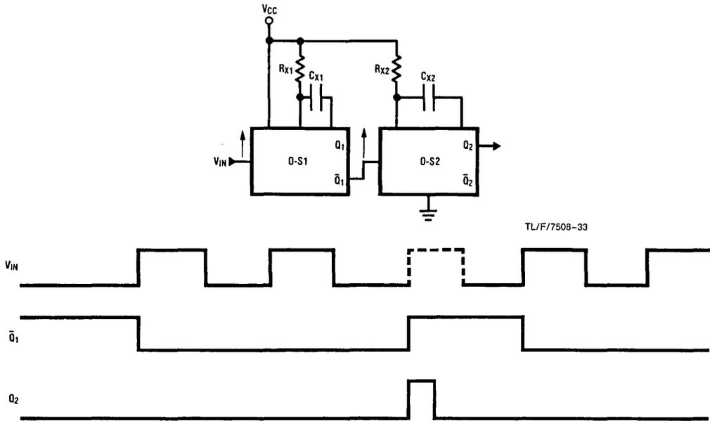
FIGURE 13. Missing Pulse Detector (Retriggerable Device Required)
