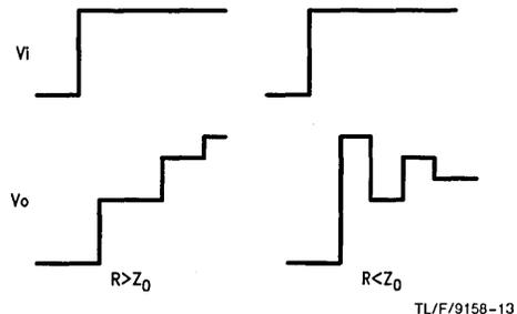
FIGURE 13. Waveforms for Improperly Terminated Transmission Lines
