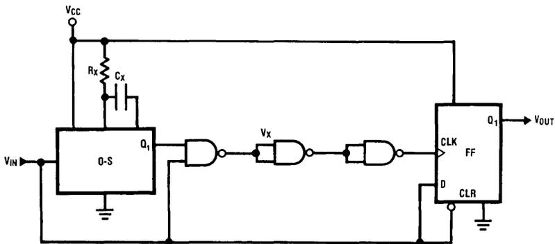
FIGURE 14. Pulse Width Detector
