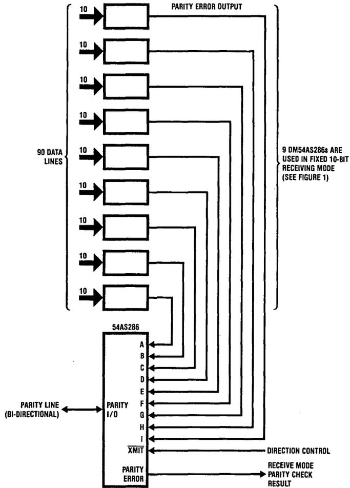
Note: Parity format in this configuration is "odd parity"
