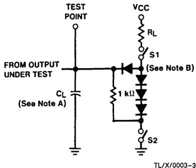
**Note A:**  $C_L$  includes probe and jig capacitance.
