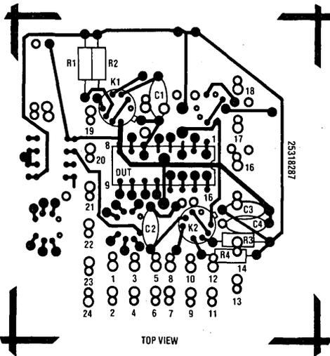
FIGURE 6a. AC Test Adapter
