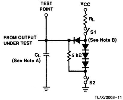
**Note A:**  $C_L$  includes probe and jig capacitance.
