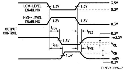
**Note:** All input pulses are supplied by generators having the following characteristics: frequency = 1 MHz, Z<sub>OUT</sub> = 50Ω, t<sub>r</sub> = t<sub>f</sub> = 2 ns.
