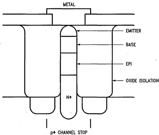
FIGURE 11. Cross Sectional View of Oxide Isolated Transistor
