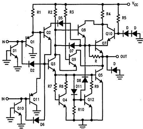
FIGURE 5. AS00 Schematic
