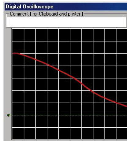
Figure 5 - Simulated delay at C_{load} = C_{REF} . Scope settings are 0.5V/div and 200 ps/div. V_{out} = V_{MEAS} at T_{CREF} = 1.20 ns.
