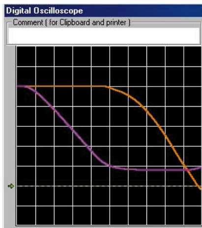
Figure 6 - Simulated delay with 6" transmission line and one receiver. Scope settings are 0.5V/div and 200 ps/div. V_{out}=V_{MEAS} at T_{VM}=0.7 ns, V_{in}=V_{IL}=0.8 V at T_{in}=1.7 ns, and T_{pin-to-pin}=T_{in}-T_{VM}=1.7-0.7=1.0 ns.
