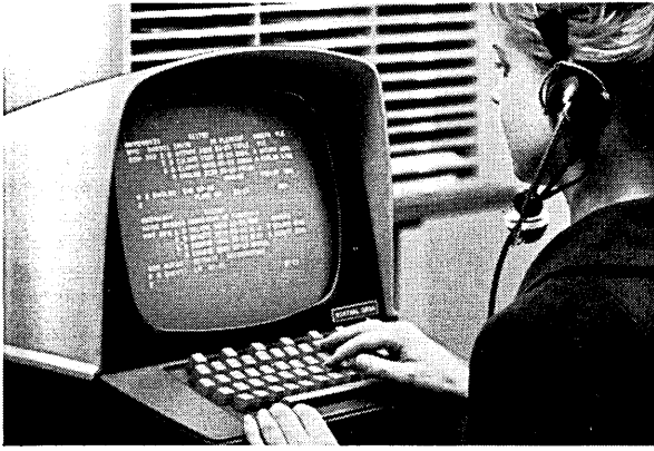
CONTROL DATA 210 Visual Display Unit . . . lets you query the central computer remotely; read out answers instantly on video screen. Up to 63 such units can share a single computer.
