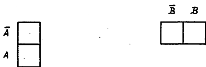
(a) Each square designated by the corresponding variable in direct or complemented form according to its state
