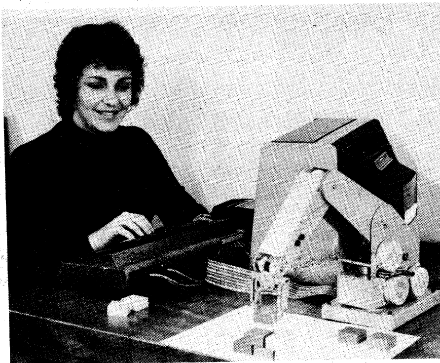
Microbot's MiniMover 5, shown above interfaced to Radio Shack's TRS-80, will demonstrate at the Computer Faire that it is armed to grasp the situation at hand.
