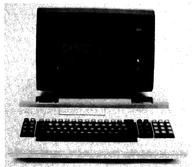
The Model 3101 signalled IBM's entry into the ASCII terminal market. Human engineering features on the 3101 include a tilt and swivel monitor, a concave contrast-enhancing screen filter, and a detachable keyboard. The 3101 is available for purchase only, and prices begin at $1,295. Quantity discounts are also available.
