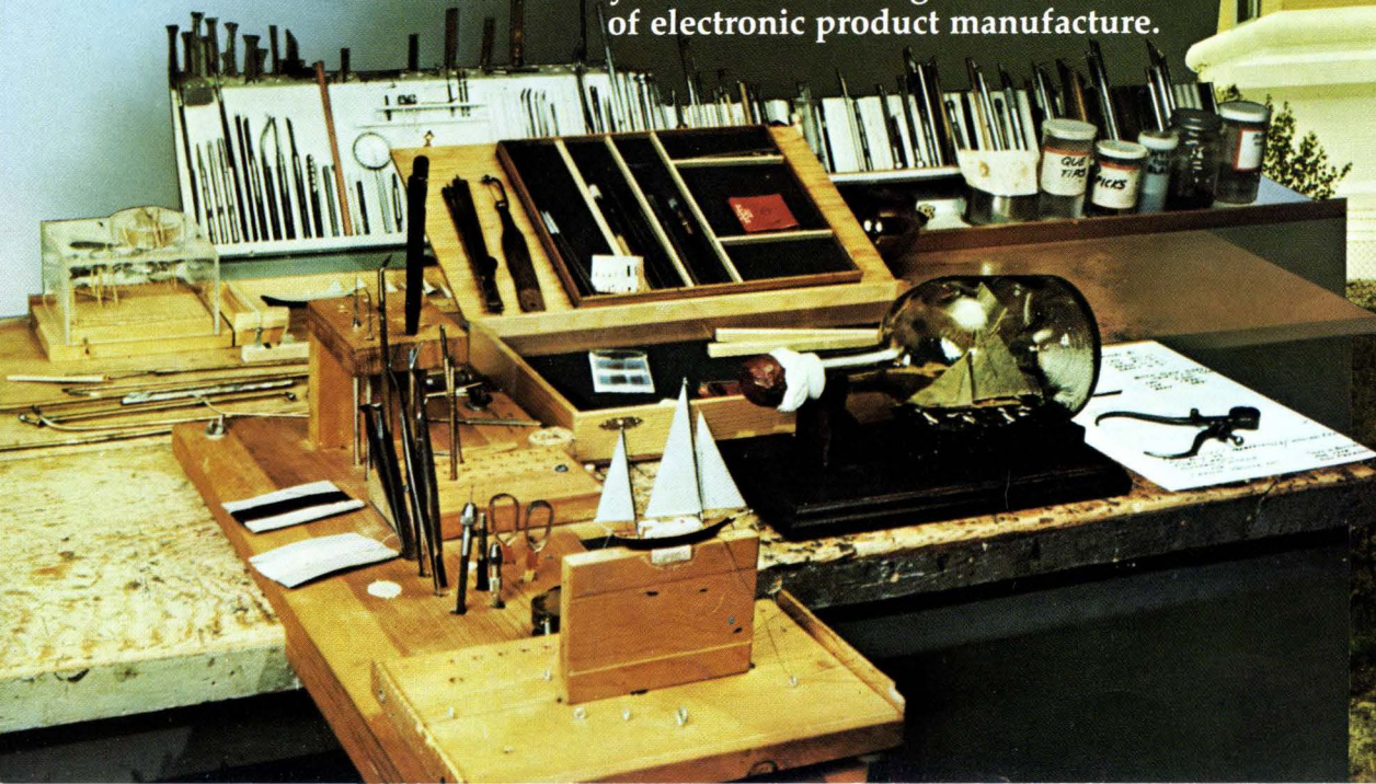
The age-old art of building ships in bottles demands, even today, the maximum of craftsmanship. As many as 100 collapsible parts with threads attached make the impossible possible inside the glass prison.
