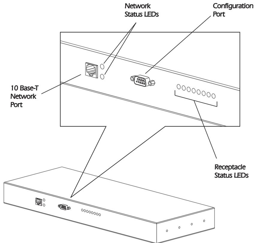
Figure 1: MasterSwitch Front Panel
