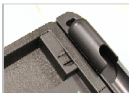
A4 spacer inserted on the left side of the notepad slot.
